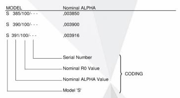
Each thermometer is identified with coding information and serial number. However, when ordering it is recommended that the full Model number is used. SDL would be pleased to quote to Customers requiring special thermometers, a high temperature capability, alternative characteristics or mechanical designs.
